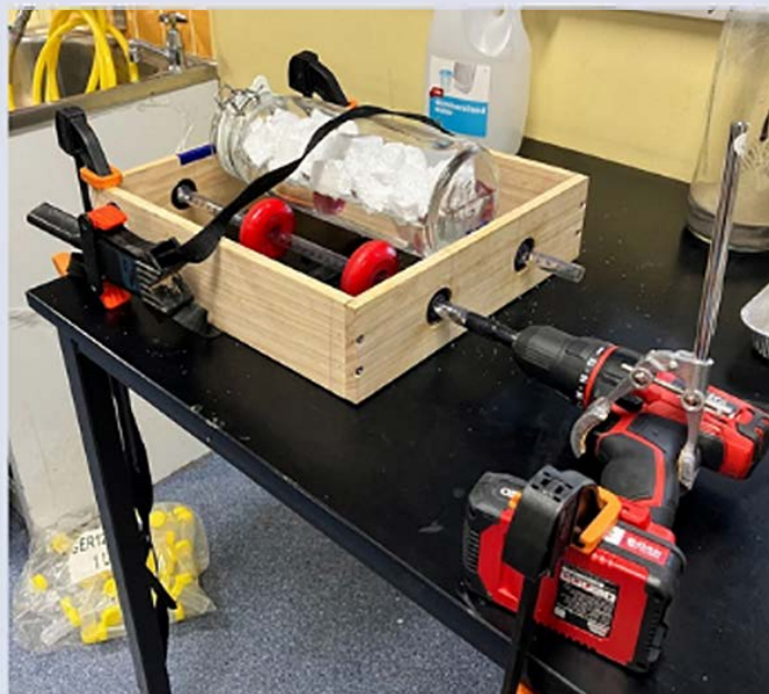
Figure 1. Spinning barrel apparatus based on rock tumbler design used to simulate the surf zone along a sandy beach coastline and open ocean in this investigation.
