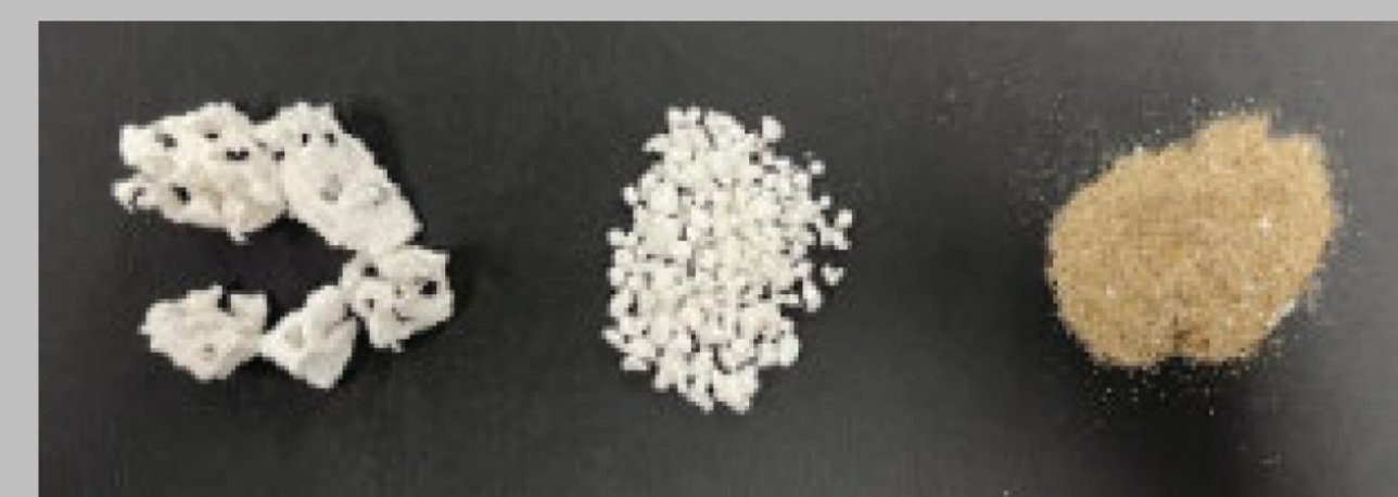
Figure 7. Photographic evidence of PS consumption from Test colony. Left to right progression of boring in large PS pieces and progressive fragmentation to smaller pieces mixed with frass.
